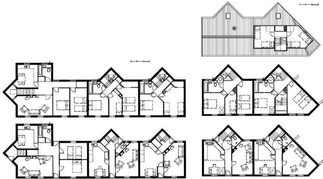
Flat and house plans for Barrow-in-Furness [left]. A later variant [right] has the same principles, of non-overlooking of the back gardens, applied to a larger 4-bedroom house. The 'mitre' allows the terrace to turn a corner, either 45° or 90°. Optimum house width and depth was used in order to maintain historic densities.
