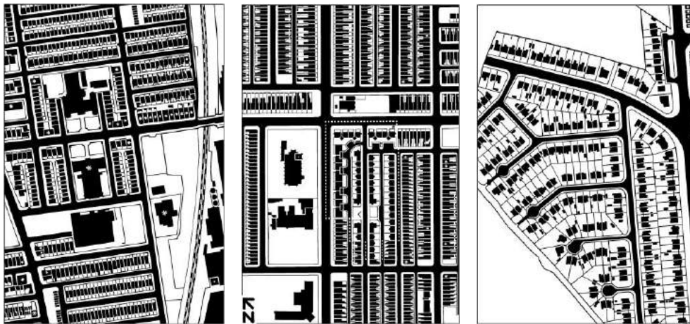
Comparative plans, to the same scale, of Saltaire [left], Hindpool [centre] and pre-war semis [at a relatively high density] in Denton, Greater Manchester [right]. The asterisks indicate shops or communal facilities. The area within the dotted line in the central plan contains 79 houses and flats built in 1985.
